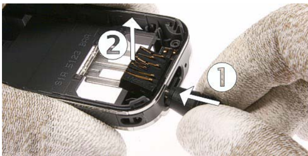
19.) Press out the Easy Flash Connector by using the DC-plug.
